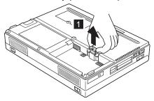
b) Install the battery pack as shown 2 , sliding the battery-pack lock toward the rear of the computer 3 .
