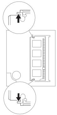
b) Remove the DIMM.
