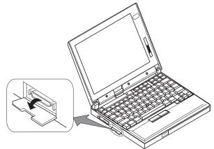
**3** Attach the cable to the external diskette drive 1 ; then to the external-diskette-drive connector on the side of the computer 2 .
