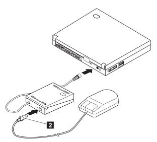
Attaching an External Numeric Keypad or a Mouse
