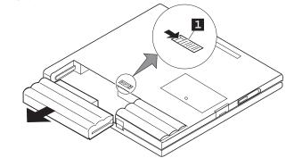
**4** Align the guides on the fully charged spare 2 with the ones on the computer 3 ; then slide the battery pack into the computer.
