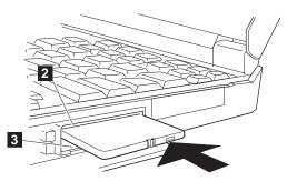
**4** Press the PC Card firmly into the connector until the eject button 4 pops out. Then, pull the eject button out slightly and fold it to the left.
