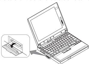
3 Attach the cable to the external diskette drive; then to the external-diskette-drive connector on the side of the computer.
