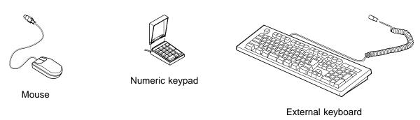
You can attach an external numeric keypad, a mouse, or an external keyboard directly to the external-input-device connector ( on the rear of the computer.
