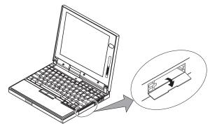
$oldsymbol{3}$  Insert the PC Card into the appropriate slot according to your PC Card type.
