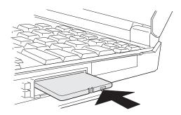
**4** Press the PC Card firmly into the connector until the eject button pops out. Then, pull the eject button out slightly 1 and fold it to the left. 2.
