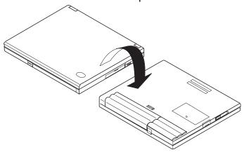
**3** Slide the battery pack latch 1; then slide the battery pack toward the front of the computer and remove the battery pack.
