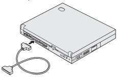
**3** Connect the AC Adapter to the computer's power jack (at the rear of the computer) in the order shown.
