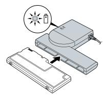
**4** When the charging indicator stops blinking and stays on, remove the battery pack from the battery charger.
