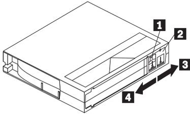
The front of the cartridge has an orange **write-protect** indicator 1, and a **write-protect** switch 2 to prevent accidental erasure. Slide the switch to the right to write-enable 3 or to the left to write-protect 4. You can change the **write-protect** switch before or after inserting the tape. If you change the write-protect switch while the tape is inserted, there is a delay of a few seconds before the **Write Protect** indicator on the tape drive changes.
