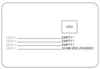
Refer to the graphic on screen to determine if the DIMMs passed or failed the extended memory test. To locate the memory socket positions the system board, see "System Board" on page 96.
