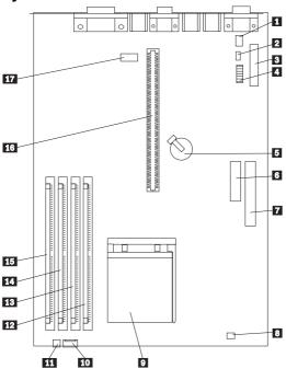
1 Auxiliary power connector 2 CMOS clear (password) jumper 3
